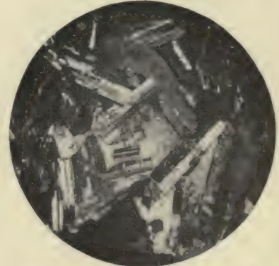
FIG. 4.—Monzonite texture. The orthoclase fills the interstices between the plagioclase laths. Polarized light.
